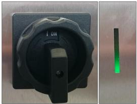
To turn the dehumidifier on, press the button on the left of the main switch. Press the button again to turn the dehumidifier off.
