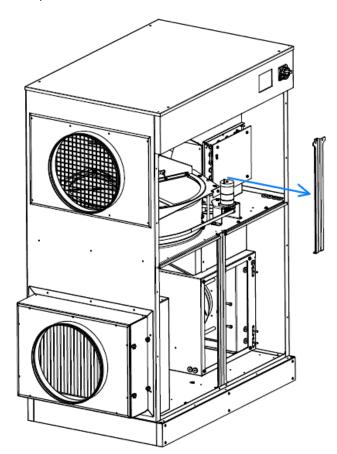
The next step is to remove the top rotor plate. The top box is connected to the heating box via. a flexible hose attached by metal bands like those on the rotor. The flexible hose has two layers of insulation, first a layer of Rockwool with a second layer of Armacell insulation on the outside.
