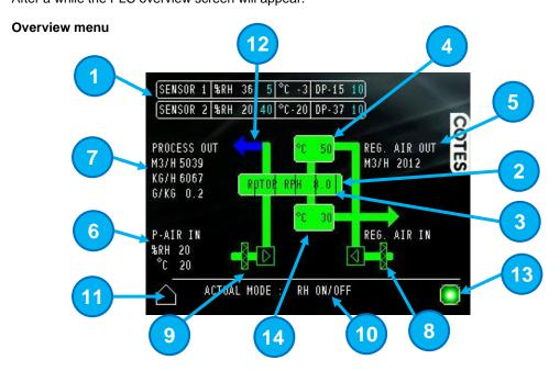
Actual measurement and target value for % relative humidity and temperature – within the space concerned (as registered by external sensors that are not part of the dehumidifier).
