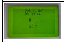
Fill in the correct values in the order: hours/minutes/seconds. To "jump" from hh to mm to ss, press the "arrow RIGHT" next to the "OK" button. To leave the menu, press simultaneously "SHIFT" and "UP arrow".
