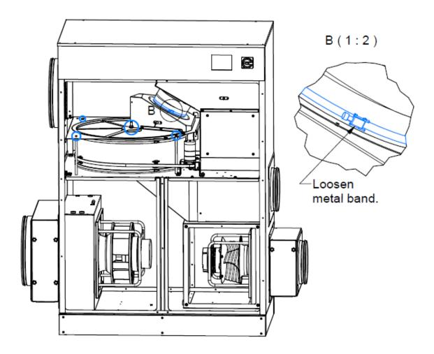
• With the rotorshaft removed, the flex hose free, and the distancepices loosened, the top rotor plate can now be removed, exposing and giving easy access to the rotor.
