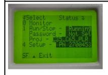
Press button "1" to return the controller to run mode. Before You choose Run mode please be sure that the On/Off button on front panel of the machine is OFF! Otherwise the machine will start operating immediately after you select Run mode!
