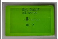
Enter the correct date values in the order: day/month/year. To "jump" from dd to mm to yy, press the "right arrow" next to the "OK" button. To leave the menu without saving press simultaneously "SHIFT" and "UP arrow".
